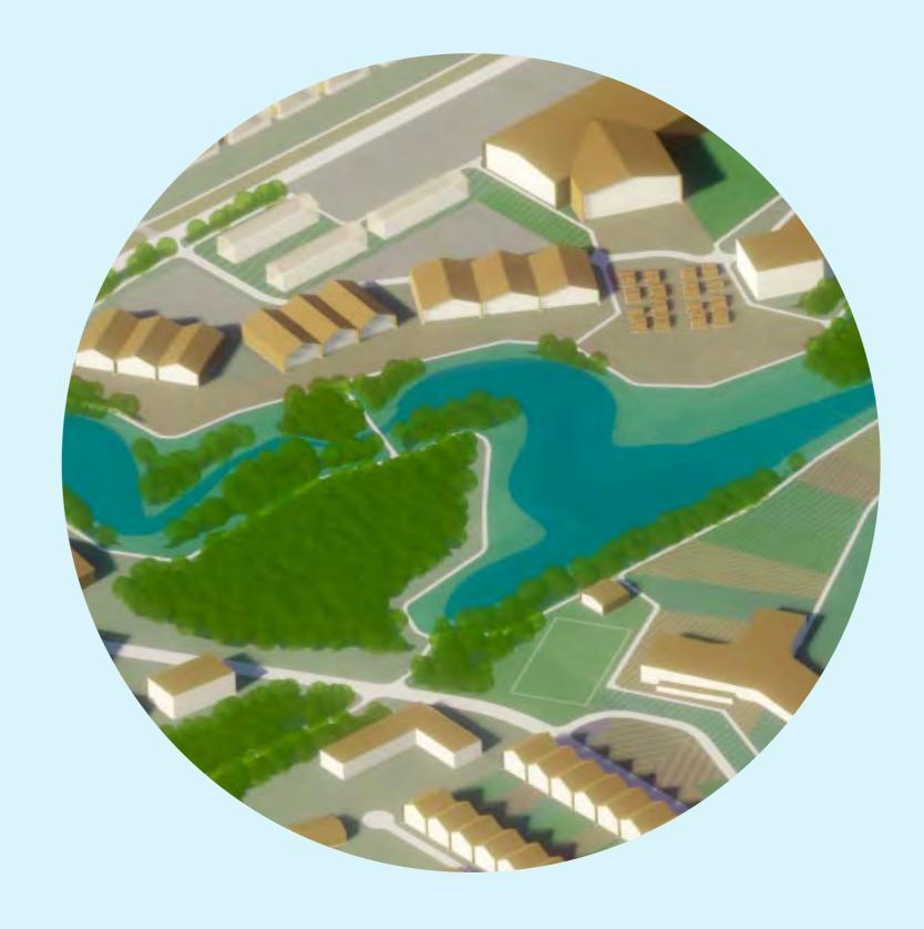
The wetland anchors the north end of the Central Commons and provides a buffer between the commercial uses to the north and the agricultural production to the south. A naturally-occurring feature, it has been developed into a functioning storm pond, a rich ecosystem, and a beautiful recreational amenity. Trails surround the wetland, and main roads cross its threshold over beautiful bridges. PROPRIETARY & CONFIDENTIAL
